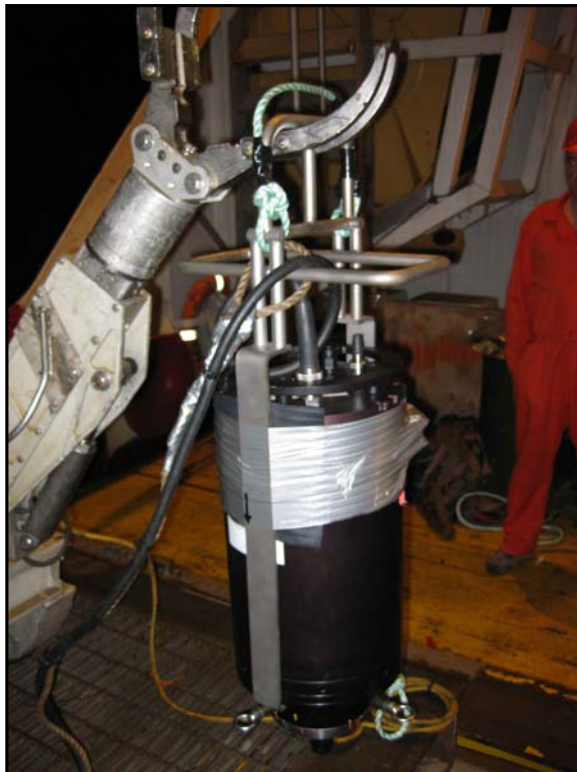
Figure 3: C-PINS installed as deployed in 5 function manip.
