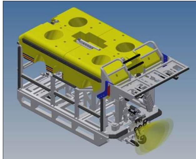
A single RS232 is required for the management and configuration of 3D Recon. A GB Ethernet port is required for the image data. All Power, serial communications and the imaging data is connected via a single PBOF cable to the ROV (RTS Mux or Innova Mux). The GB Ethernet connection is available as copper. Power requirements are 24Vdc 150W.
